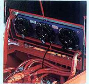
Hydraulic/brake oil cooling system
